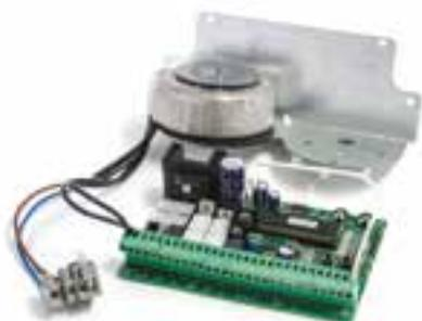
12VDC logic board for 2 leaves swing gate openers, transformer and receiver for 120 codes
